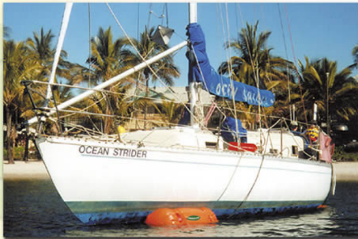
Photo: 7 ton yacht lifted 0.3m (1ft) by four (4) EL500s to reduce the draft
